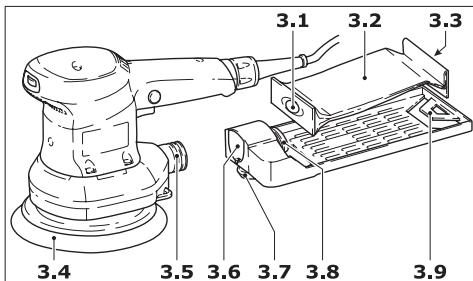
The machines are fitted with inbuilt extraction as standard. The sanding dust is extracted through suction openings in the sanding base (3.4) and trapped in the turbo-filter (3.2).
